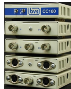
Front panel Rear panels: Composite video Composite video with GPI S-Video S-Video with GPI
